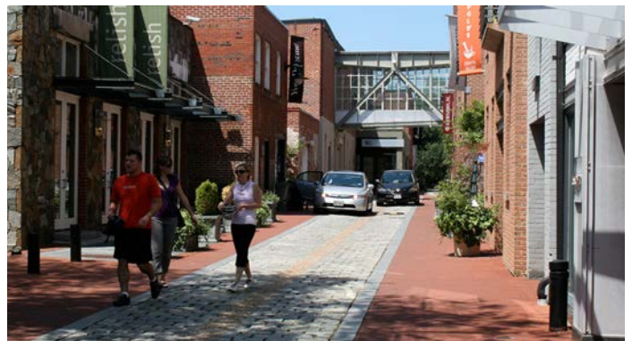
Williams and Eagle River Streets shall be designed as "woonerfs" - or shared streets - where cars, pedestrians, and bikes all share the space equally and the street is designed so cars travel at very low speeds.
