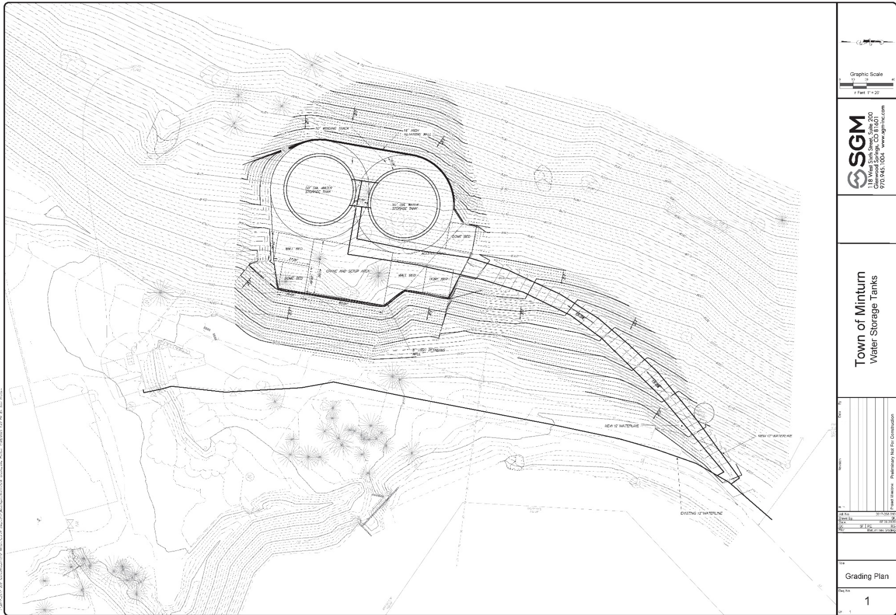
Figure 4: Water Storage Tanks Site Plan
