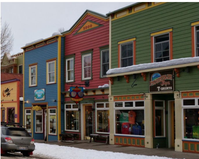
The street level of a building facing Main Street shall include a minimum of 70% transparency, have an entrance every 25-feet and be designed to provide visual interest.
